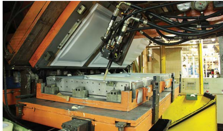
Refrigerator foaming process
